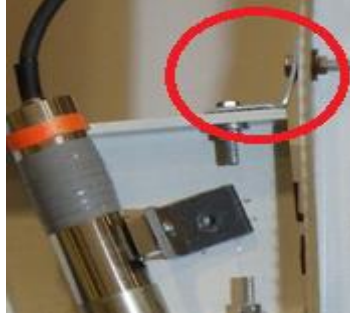
Figure 10 - Top cleat plastic deformation.
